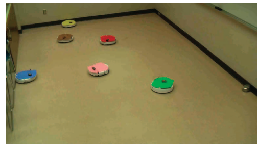
Fig. 7. Experimental setup consisting of six iRobot creates equipped with epic motes.
