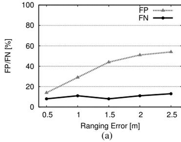
Fig. 4. Effects of range error on system performance ( $NR=12$ ,  $TH=[4,5,9,9,13]$ ).
